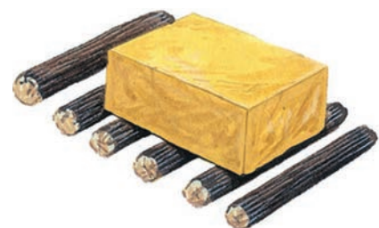
Block of stone being moved on wooden rollers
